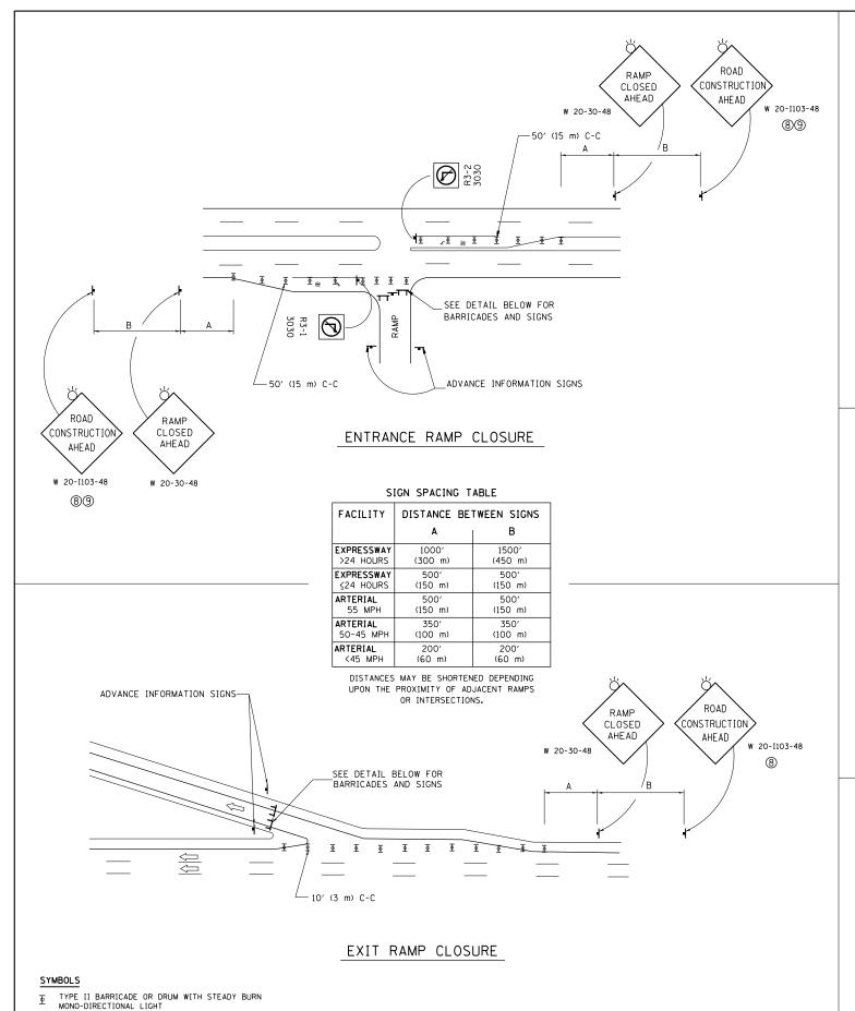
TYPE III BARRICADE WITH 2 FLASHING LIGHTS
