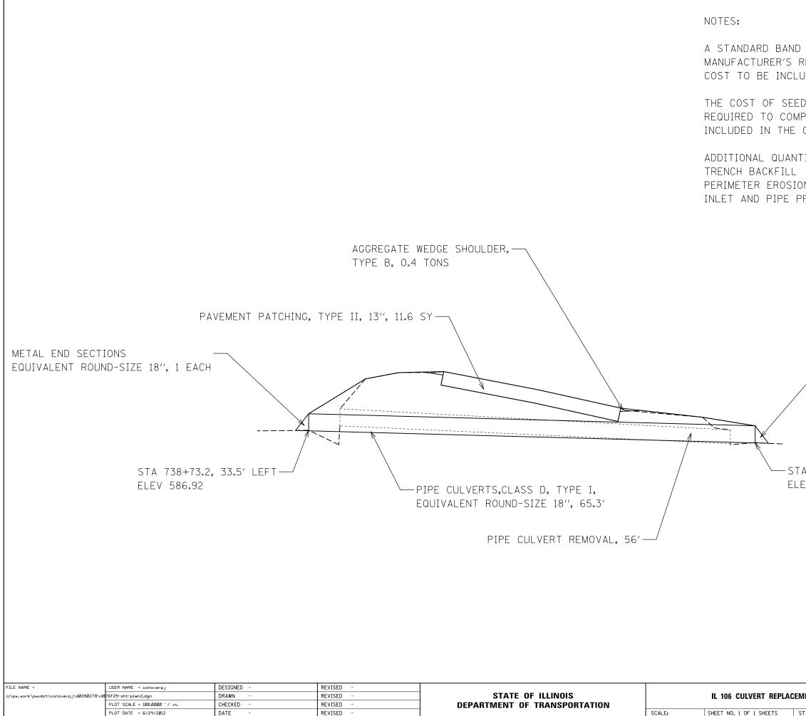
A STANDARD BAND ANGLE CONNECTOR SHALL BE USED PER MANUFACTURER'S REQUIREMENTS TO CONNECT THE PIPE CULVERT. COST TO BE INCLUDED IN THE CULVERT PAY ITEMS.
