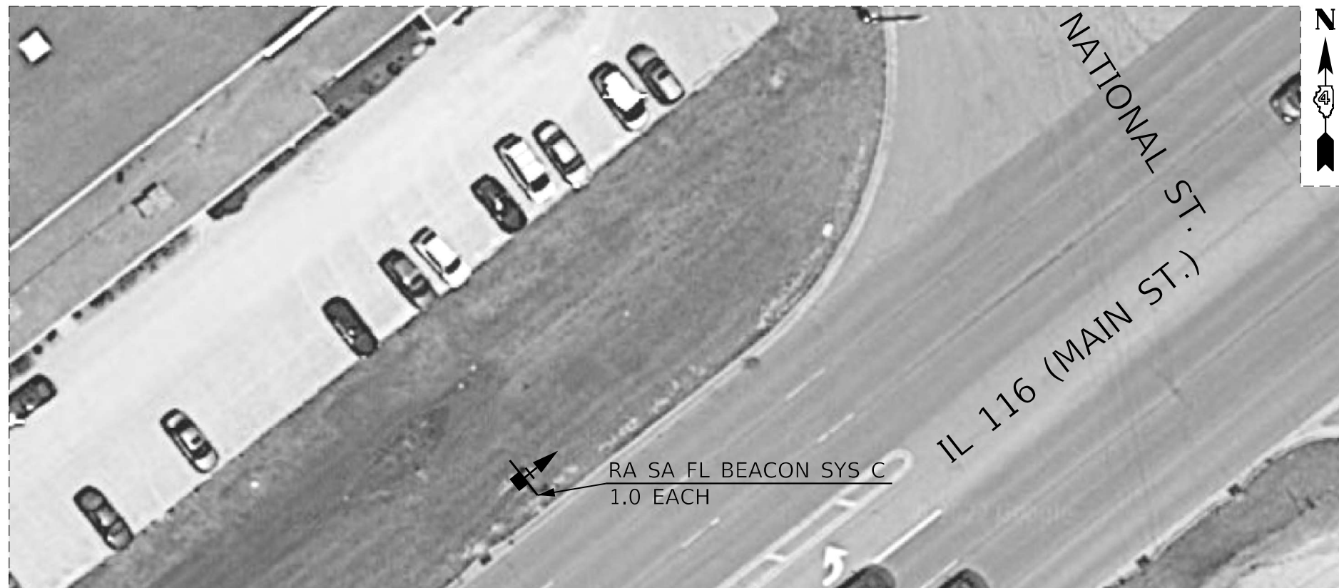
RADIO ACTIVATED SOLAR ADVANCE FLASHING BEACON SYSTEM (COMPLETE) LOCATION B
