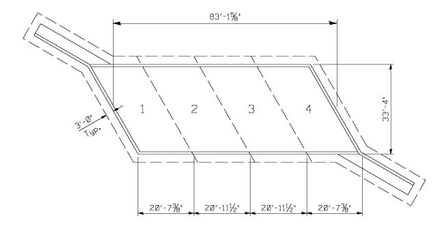
Figure 1: Sections under Proposed Culvert
