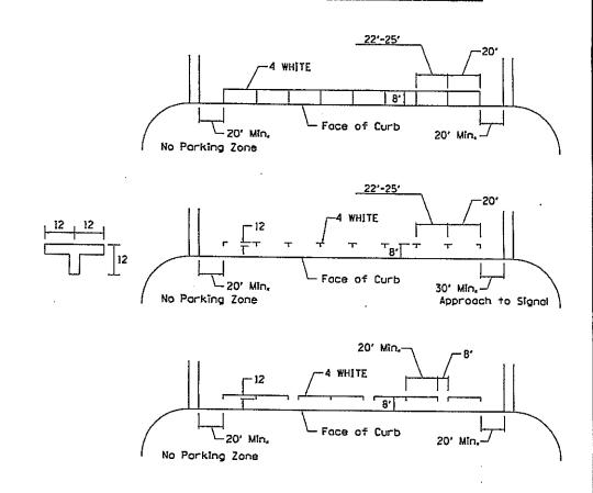
TYPICAL PAVEMENT MARKING FOR TWO LANE SECTION - NO PASSING ZONES
