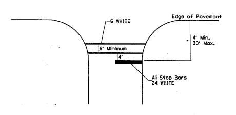
Distance to the nearest edge of the intersecting roadway in the absence of a marked crosswalk.
