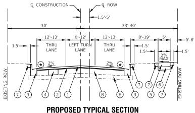
★ FINISHED PAVEMENT SURFACE SHALL BE 1/4" ABOVE TOP OF GUTTER
