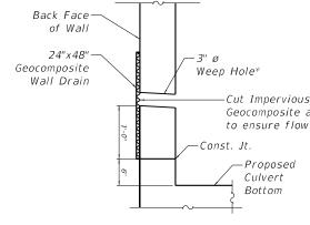
WEEP HOLE DRAIN DETAIL
