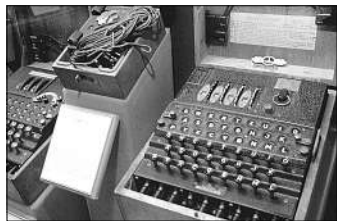
This is the four-rotor Enigma machine, once used by the German U-boat crews, that Alan Turing cracked.
