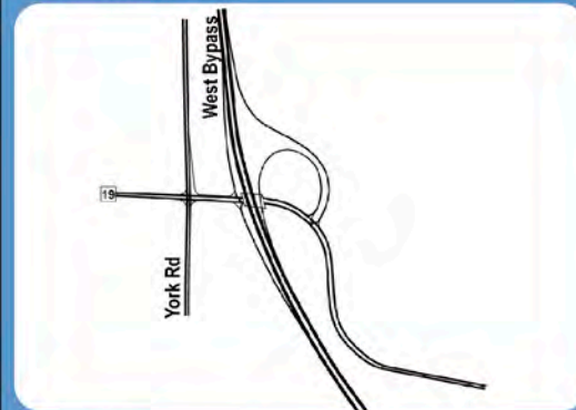
Modified diamond interchange with single loop ramp
