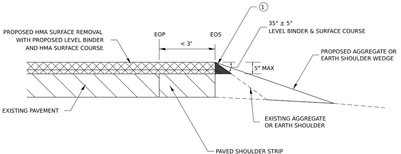
**MILLING: WITH ADJACENT SHOULDER FLUSH WITH OR HIGHER THAN MILLED SURFACE**
