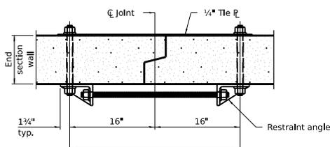
1"  $\varnothing$  Anchor rods with 2 1/4" x 2 1/4" x D" R washers installed in 1 1/2" dia. formed holes in end section walls
