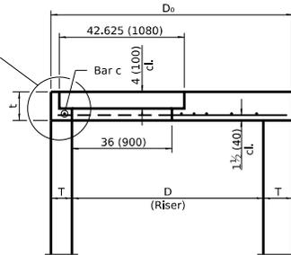
**SECTION THRU FLAT SLAB TOP**
