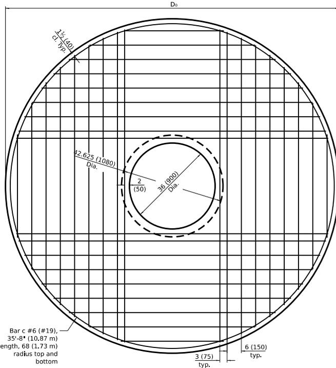
**PLAN - FLAT SLAB TOP FOR D = 10'-0" (3.05 m)**
