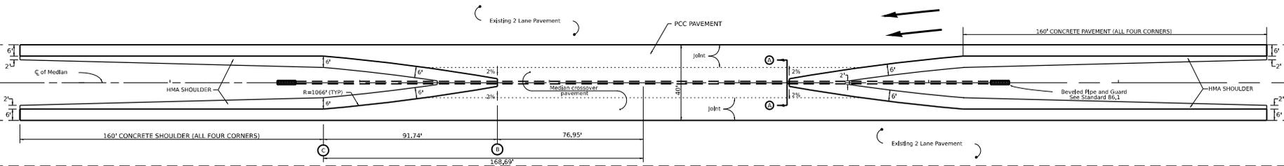
Unless otherwise specified, when the median crossover is to be removed, the Contractor shall be required to saw full-depth along the shoulder line 6' from edge of pavement. The 6' adjacent to the edge of pavement shall remain in place and be used as shoulders. The cost of Sawing shall be included in the Pavement Removal.
