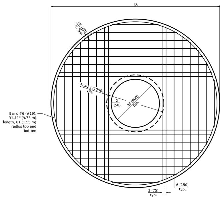
**PLAN - FLAT SLAB TOP FOR D = 9'-0" (2.74 m)**
