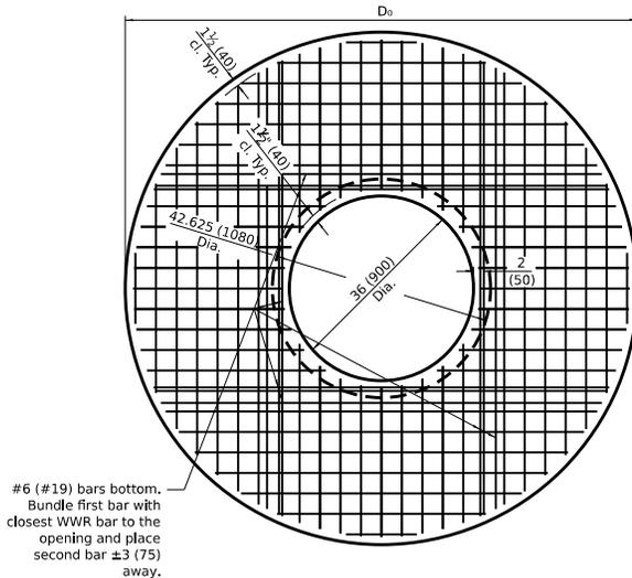
**PLAN - FLAT SLAB TOP FOR D = 7'-0" (2.13 m)**
