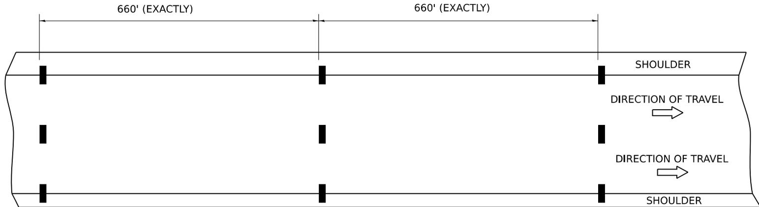
USE THERMOPLASTIC PAVEMENT MARKINGS MEETING THE REQUIREMENTS OF SECTION 782 OF THE STANDARD SPECIFICATIONS.
