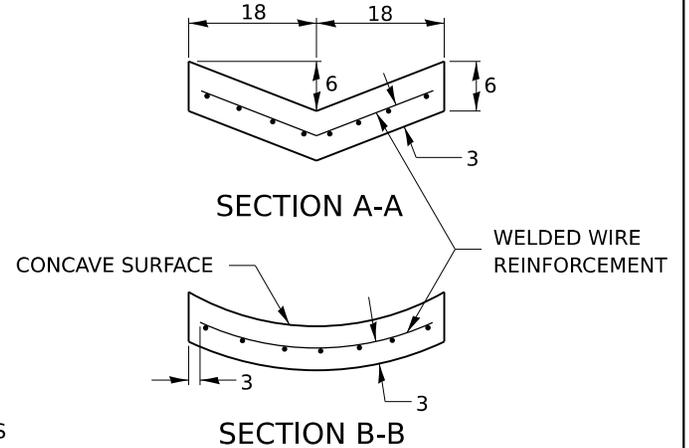
EDGE OF PAVEMENT TO SECTION A-A INCLUDING TWO CUTOFF WALLS 1.02 CU YDS
