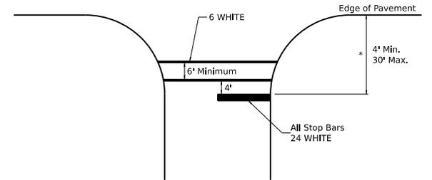
\* Distance to the nearest edge of the intersecting roadway in the absence of a marked crosswalk.
