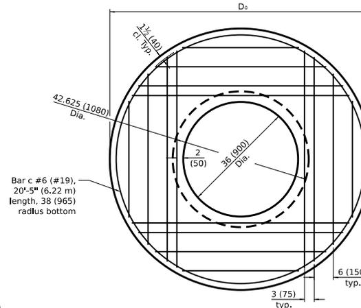
**PLAN - FLAT SLAB TOP FOR D = 6'-0" (1.83 m)**
