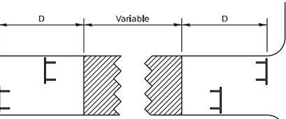
Type III Barricades and R11-4-4830 signs shall be as shown in "Road Closed to Thru Traffic" detail on Highway Standard 701901. If the distance "D" exceeds 2000' an additional set of barricades and R11-4-4830 shall be placed at each end of the work area.
