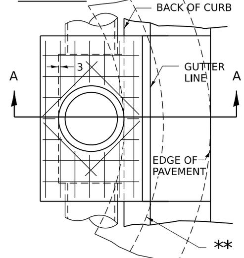
\*\*WHEN INLET IS CONSTRUCTED IN RETURN, THE TOP OF SLAB SHALL CONFORM TO THE RADIUS OF THE RETURN.
