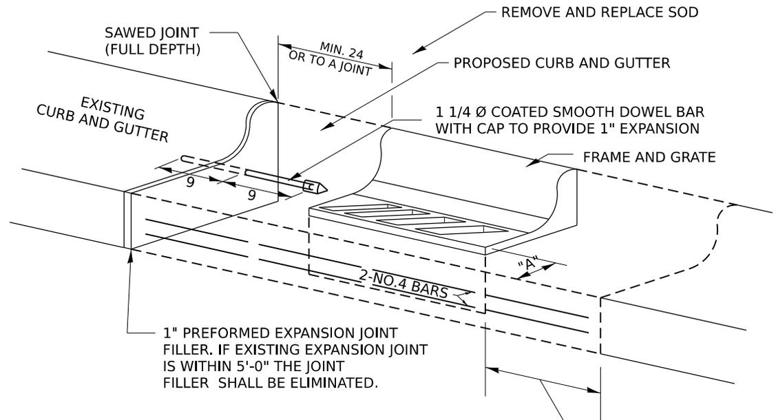
WHEN "A" IS GREATER THAN 2, 2-NO. 4 BARS SHALL BE PLACED AS SHOWN.
