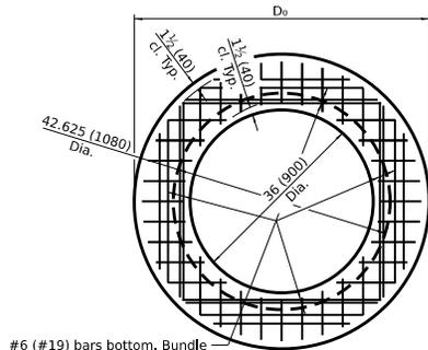
**PLAN - FLAT SLAB TOP FOR D = 4'-0" (1.22 m)**
