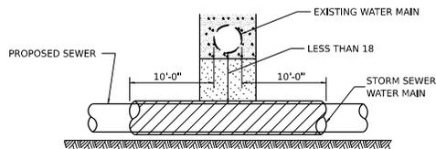
PROVIDE ADEQUATE SUPPORT FOR EXISTING WATER MAIN TO PREVENT DAMAGE DUE TO SETTLEMENT OF SEWER TRENCH
