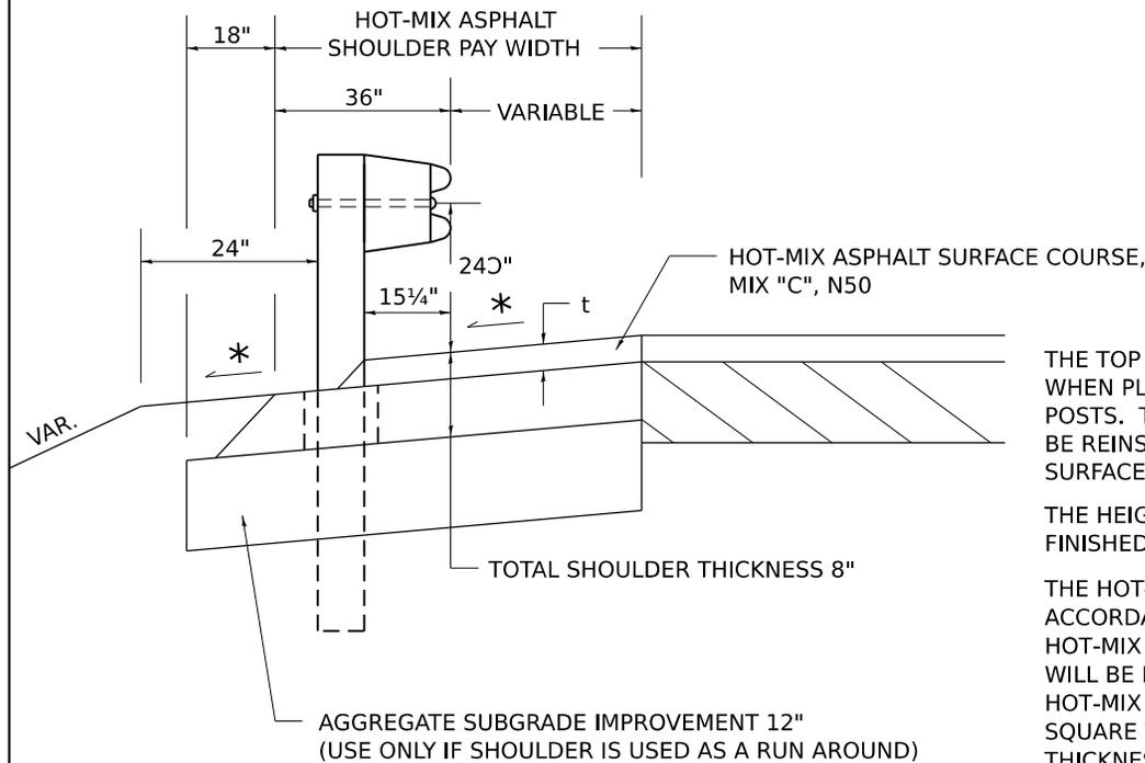
t = SEE TYPICAL SECTIONS FOR THICKNESS
