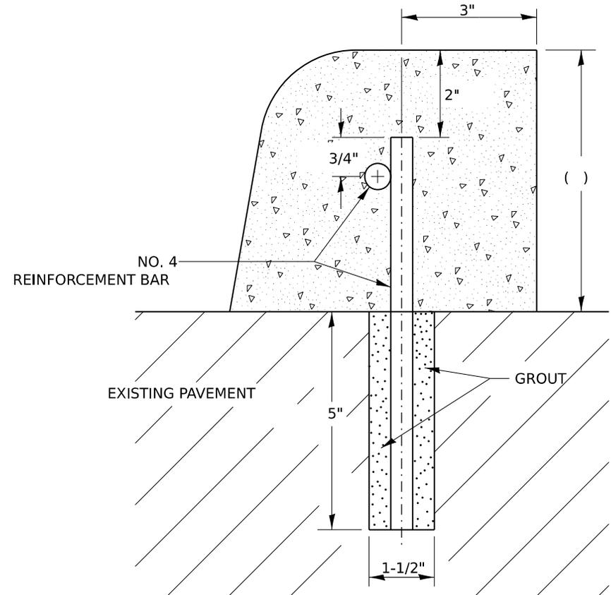
CONCRETE CURB (SPECIAL) SHALL BE CONSTRUCTED IN ACCORDANCE WITH SECTION 606 OF THE STANDARD SPECIFICATIONS, SUPPLEMENTAL SPECIFICATIONS, STANDARD 606001 AND THIS DRAWING.
