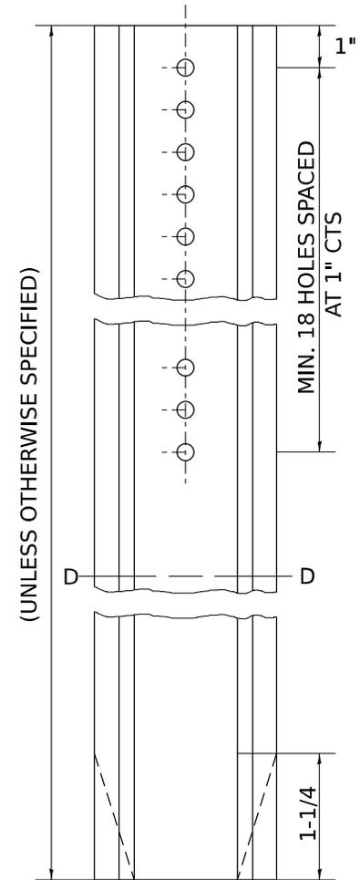
DELINEATORS SHALL BE INSTALLED ACCORDING TO STANDARD 635001 EXCEPT THAT THE POST SHALL BE ROTATED 180°. THE POST WILL HAVE THE WIDE SIDE FACING TRAFFIC AND THE DELINEATOR ATTACHED AS SHOWN ABOVE.
