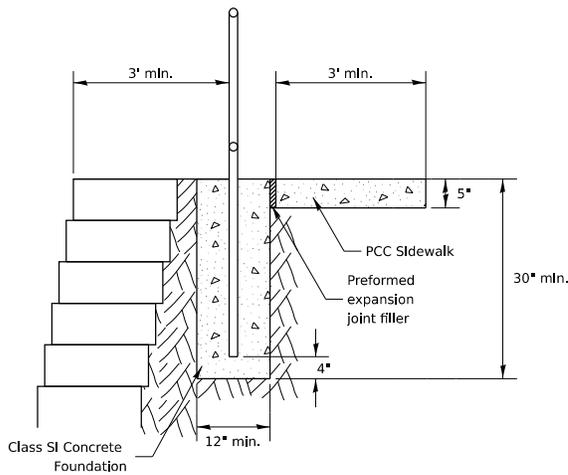
**PIPE HANDRAIL, SPECIAL - FOR RETAINING WALL**
