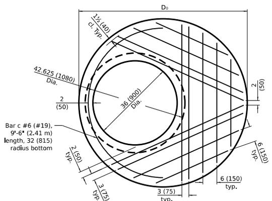
**PLAN - FLAT SLAB TOP FOR D = 5'-0" (1.52 m)**
