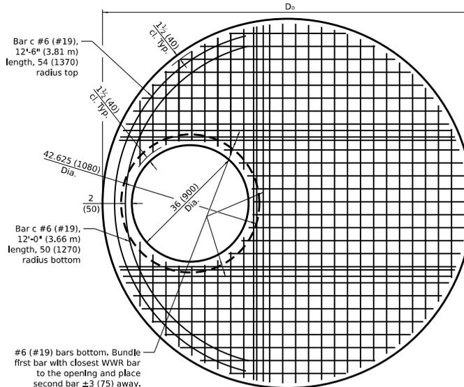
**PLAN - FLAT SLAB TOP FOR D = 8'-0" (2.44 m)**
