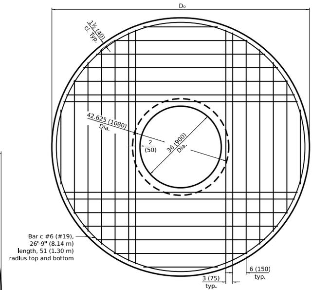
**PLAN - FLAT SLAB TOP FOR D = 8'-0" (2.44 m)**
