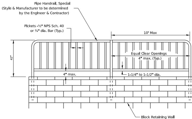
**PIPE HANDRAIL, SPECIAL - FOR RETAINING WALL**
