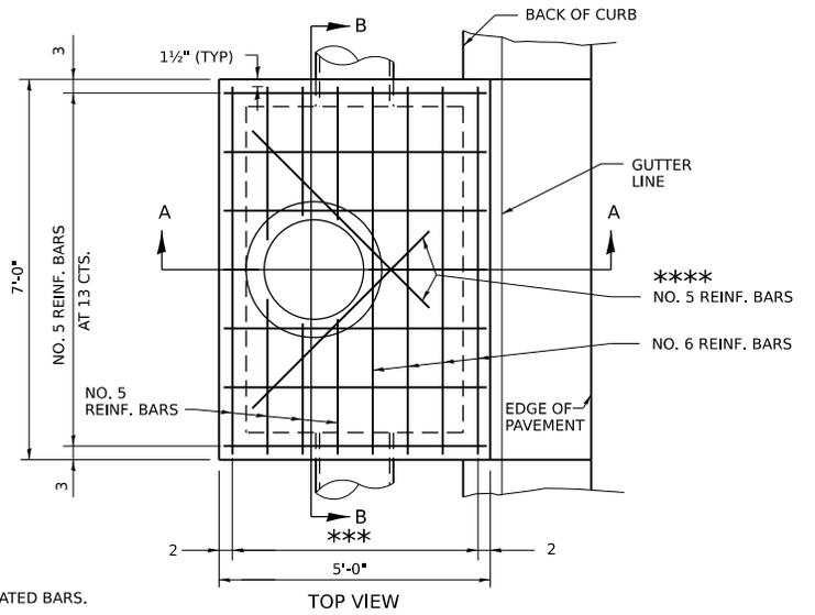
\* THE WALL ADJUSTMENTS SHALL BE MADE WITH CONCRETE BUILDING BRICK OR CLASS SI CONCRETE.
