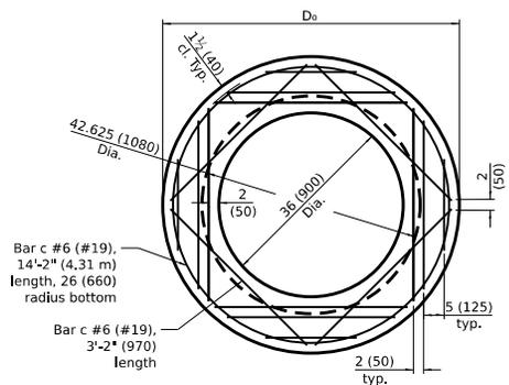
**PLAN - FLAT SLAB TOP FOR D = 4'-0" (1.22 m)**
