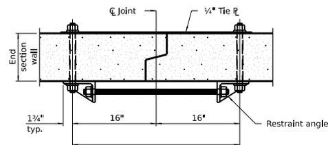
1" Ø Anchor rod with 2 1/4" x 2 1/4" x D" washers installed in 1 1/8" dia. formed holes in end section walls
