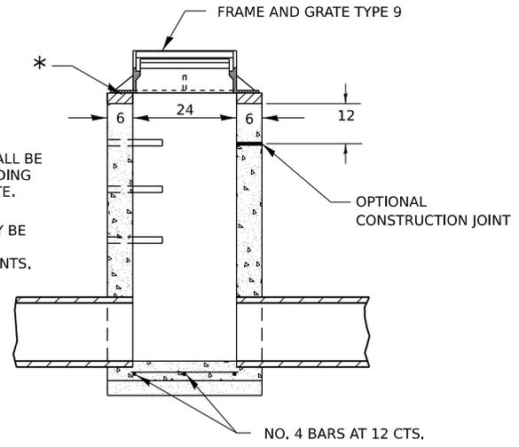
\* THE WALL ADJUSTMENTS SHALL BE MADE WITH CONCRETE BUILDING BRICK OR CLASS SI CONCRETE.
