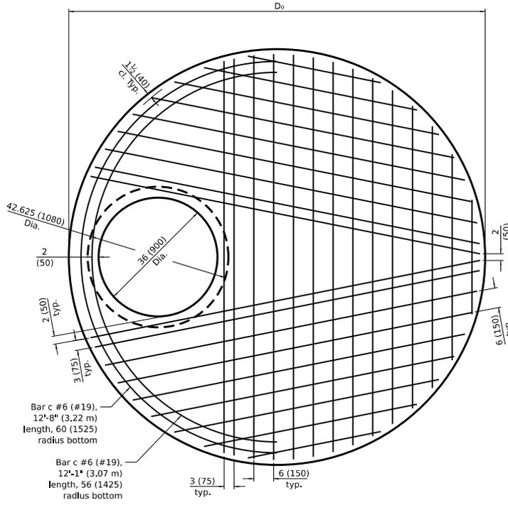
**PLAN - FLAT SLAB TOP FOR D = 9'-0" (2.74 m)**
