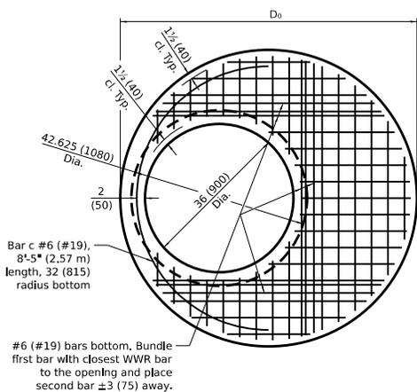
**PLAN - FLAT SLAB TOP FOR D = 5'-0" (1.52 m)**
