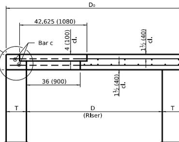
**SECTION THRU FLAT SLAB TOP**
