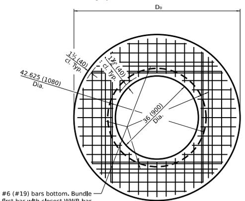
**PLAN - FLAT SLAB TOP FOR D = 5'-0" (1.52 m)**
