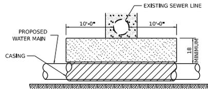
CASING SHALL BE CAST IRON WITH AN INSIDE DIAMETER 2" LARGER IN DIAMETER THAN ENCASED PIPE OUTSIDE DIAMETER WITH BOTH ENDS OF CASING SEALED
