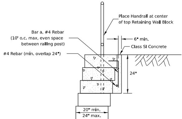
**PIPE HANDRAIL, SPECIAL - FOR RETAINING WALL**
