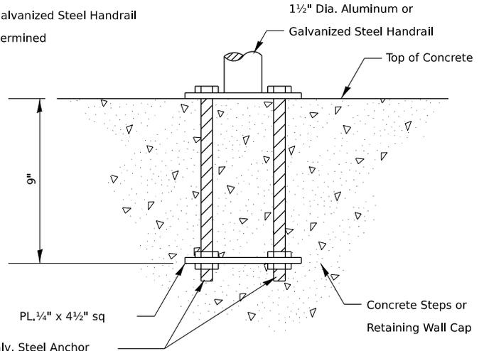
3/4" Dia. Galv. Steel Anchor Rod Thd'd both ends with Heavy Hex Nut Washer & two Hex Nuts
