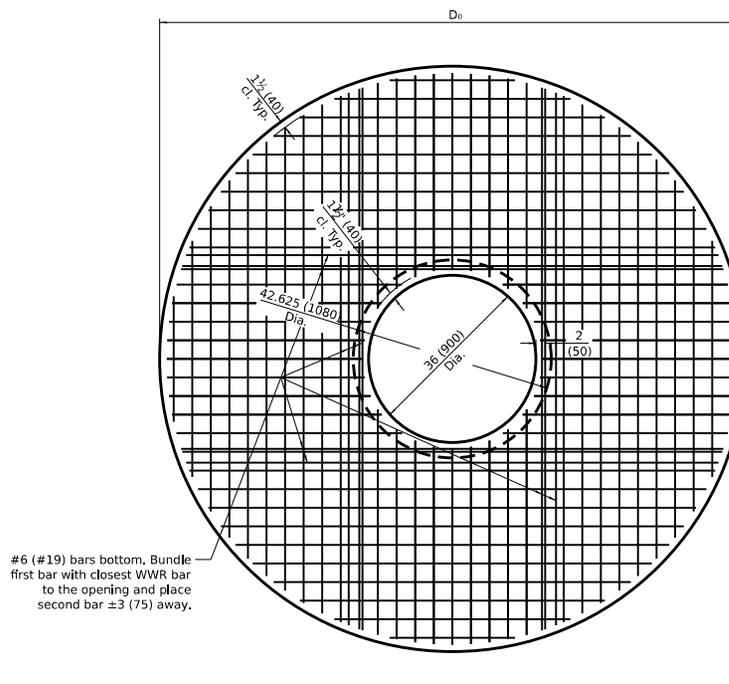
**PLAN - FLAT SLAB TOP FOR D = 9'-0" (2.74 m)**
