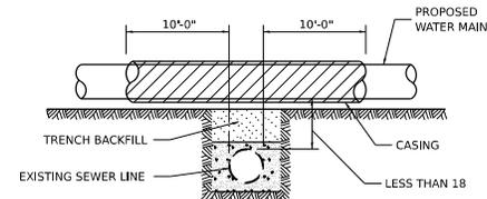
CASING SHALL BE CAST IRON WITH AN INSIDE DIAMETER 2" LARGER IN DIAMETER THAN ENCASED PIPE OUTSIDE DIAMETER WITH BOTH ENDS OF CASING SEALED
