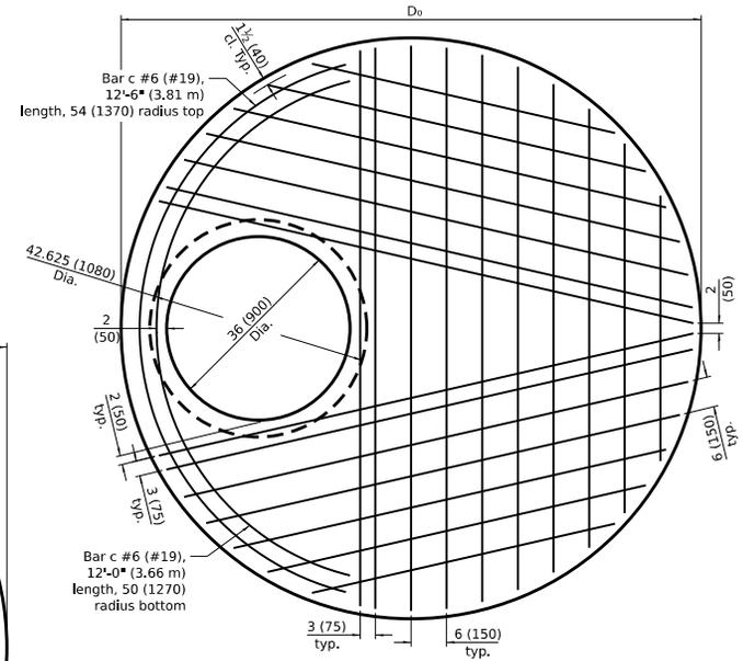
**PLAN - FLAT SLAB TOP FOR D = 8'-0" (2.44 m)**
