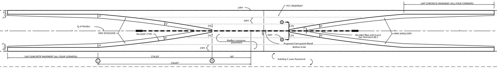
Unless otherwise specified, when the median crossover is to be removed, the Contractor shall be required to saw full-depth along the shoulder line 6' from edge of pavement. The 6' adjacent to the edge of pavement shall remain in place and be used as shoulders. The cost of Sawing shall be included in the Pavement Removal.
