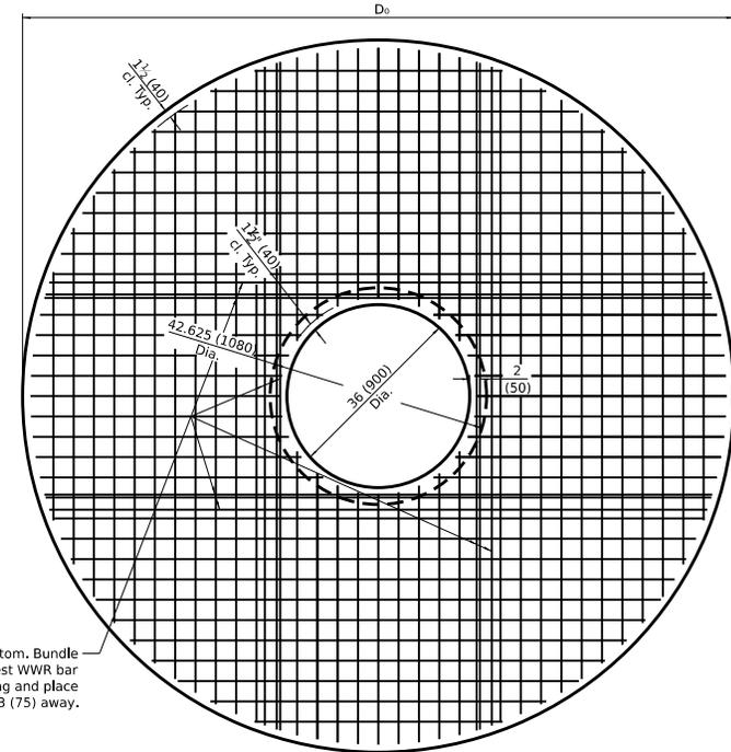
**PLAN - FLAT SLAB TOP FOR D = 10'-0" (3.05 m)**
