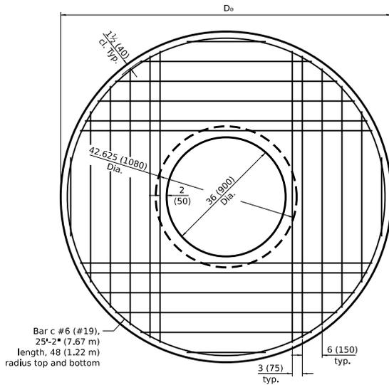
**PLAN - FLAT SLAB TOP FOR D = 7'-0" (2.13 m)**
